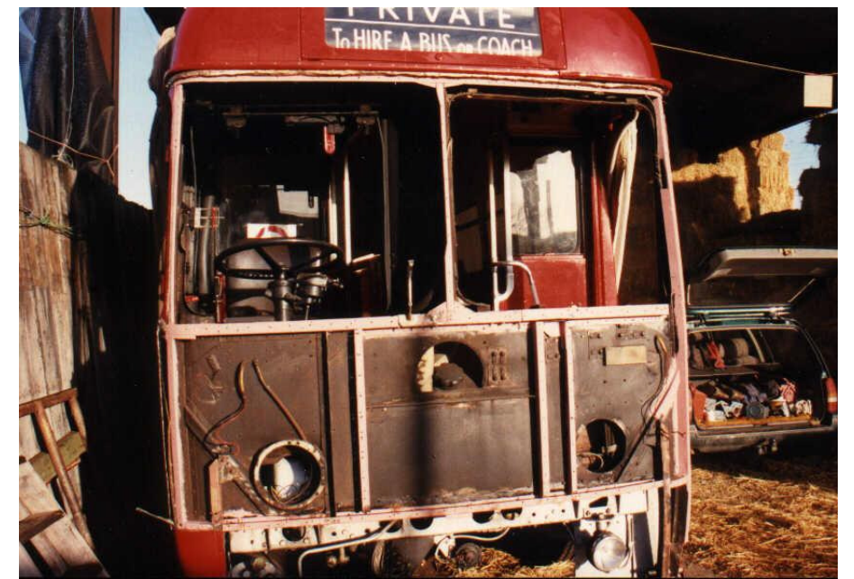
RF366 during rebuild. Photo Jim Andress
